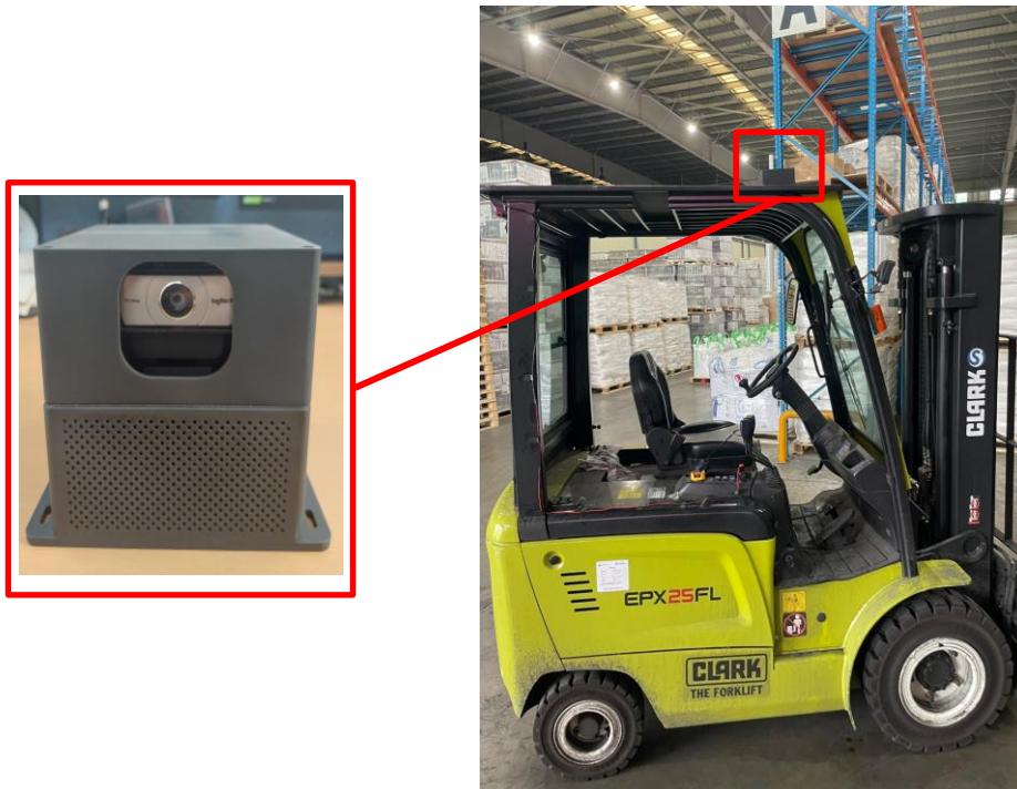
Figure 16: Camera setup on AGV
