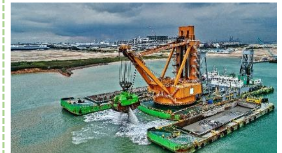
Energy Efficient Grab Dredger
